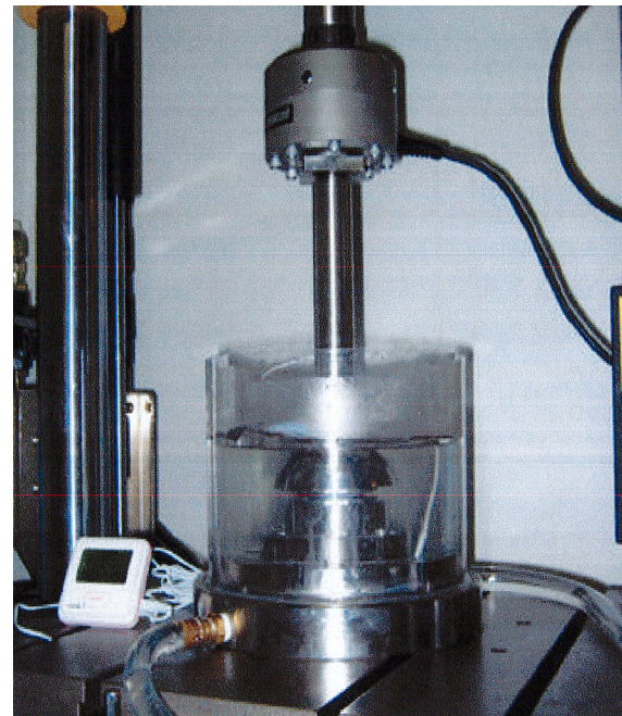
Fig. 1. Experimental setup for axial compression testing of the AxioMed® Freedom Lumbar Disc.
